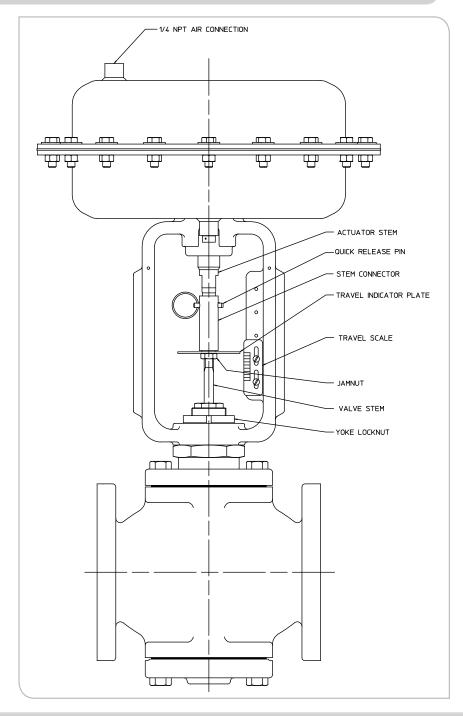
Looking down on the valve stem, the actuator can be rotated 360° to change its orientation with respect to the centerline of the valve. Changing the actuator's orientation changes the position of the travel scale, air connections, and accessories and may be necessary for clearance and accessibility in the piping.
