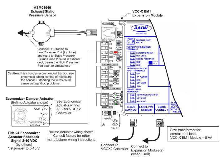
Figure 26: VCC-X EM1 Exhaust Duct Static Pressure and Economizer Actuator Feedback Wiring
