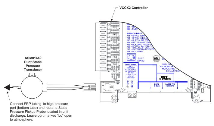
Figure 19: Static Pressure Transducer Wiring
