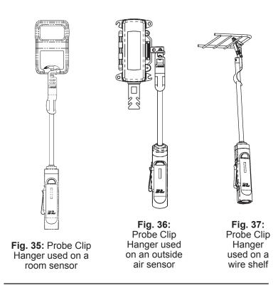
the Blü-Test probe be placed next to the outside air sensor. This may require a ladder or extension pole. Hold the Blü-Test probe in place for 3 minutes or until the reading stabilizes. The Probe Clip Hanger makes this easier by holding the probe for you (Fig. 36).
