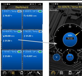
Fig. 21: Dashboard screen showing live data for 6 active Blü-Test probes.
