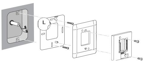
**Tip:** Before installing the power unit, it is highly recommended the labeled wires be connected to the terminals snugly according to the thermostat terminal designations (you may also refer to the picture taken in Step3). Do not overtighten.
