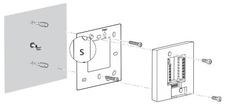
If you are mounting the thermostat on a conduit box, install the metal mounting plate enclosed with the thermostat tightly on the conduit box (making sure that the upward arrow part is placed on the top), attach the plastic trim plate to the mounting plate, and secure by screws.
