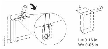
2. If needed, disconnect the cables or detach the rear module by unscrewing the screws anticlockwise. Or, if there is decoration frame, detach it as well by unscrewing the screws.
