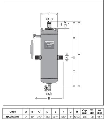
This model is ASME tagged and registered with the National Board of Boiler and Pressure Vessel Inspector and CRN registered.
