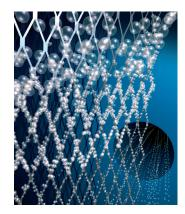
The bubbles, fusing with each other, increase in volume until the hydrostatic thrust is such as to overcome the adhesion force to the structure. They rise towards the top of the unit from which they are released through a float-operated automatic air vent valve.
