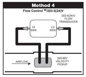
• This flow control method works from any location within the duct.
