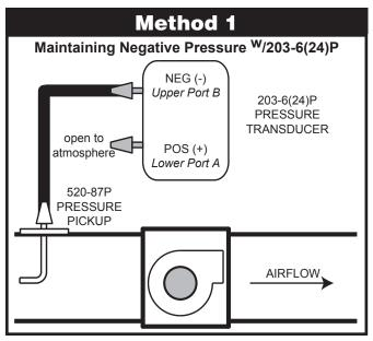
• This pressure control method works from the inlet side of an exhaust fan. The PI Interface will attempt to continuously maintain a minimum negative pressure. As the negative pressure level is reduced, the PI Interface will run the fan at a higher speed in order to maintain proper negative pressure.
