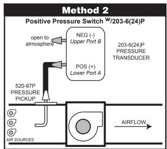
• This pressure control method works from the inlet side of an exhaust fan with other exhaust fans that randomly operate on the inlet side of the primary fan. The PI Interface will switch on the primary fan when the positive pressure builds as a result of input from multiple air sources and the transducer level exceeds PI setpoint. When the fan has reduced the pressure level sensed it will be switched off.
