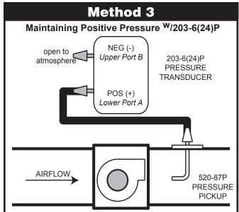
• This pressure control method works from the discharge side of a fan. The PI Interface will attempt to continuously maintain a minimum positive pressure. As the positive pressure level is reduced, the PI Interface will run the fan at a higher speed in order to maintain proper positive pressure.
