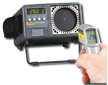
This new portable infrared calibrator provides a stable blackbody target for calibrating noncontact infrared thermometers up to 500°C (932°F). This unit features a large, temperature controlled blackbody target with a diameter of 2.25" (57mm), which offers a large field of view area for optical variations in infrared thermo-meters. The emissivity of the isothermal target is set at 0.95 (±0.02%) and the target temperature can be controlled in setpoint increments of 0.1°C.
